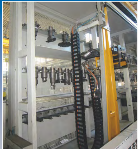
Automatic toolchanger 120 positions HSK 100 / HSK125
